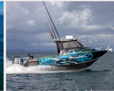
Super smooth riding hull with 20° deadrise
