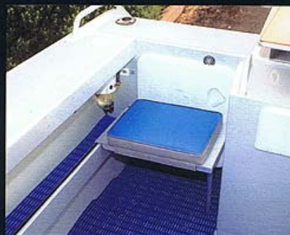
The cleverly-designed bench seats hook onto the side shelves at any point.
