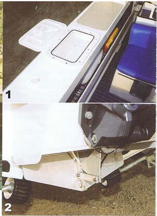
1: Stowage wells in the gunwales are useful. 2: The closing gate on the 350-litre ballast tank allowed extra weight to be retained while travelling.
